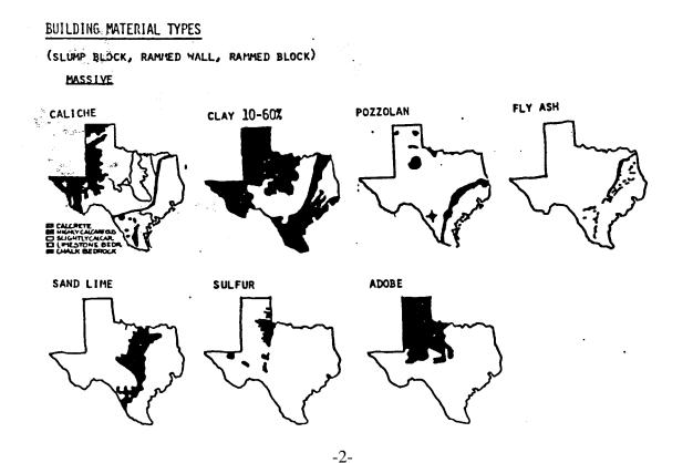
(7) <u>Adobe</u> is a sandy clay soil contain virtually no organic matter and is characteristic of arid and semi-arid climates. At its best, adobe contains about 20% clay and 80% sand, but a wide variety of mixes are used with the resulting need for higher stabilizing requirements as one deaparts from this ratio composition. Adobe makes up approximately one-third of Texas' land surface.
